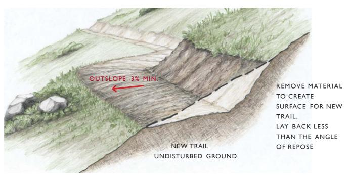
Full Bench Cut Tread Construction - Tread would be built to Forest Service standards and would include building a full bench cut trail as shown in the drawing above. Tread would be built 12"-18" wide
