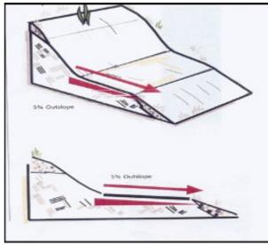
Trail tread would be outsloped 5% to allow water to flow across the tread and not down the tread, which creates erosion issues.
